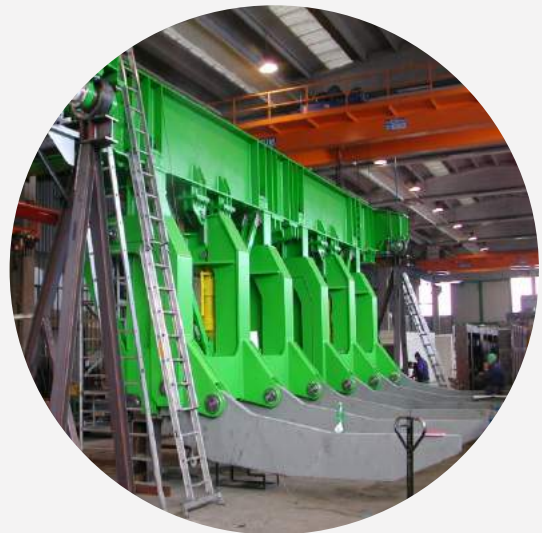
Discharging machine for walking beam furnace
